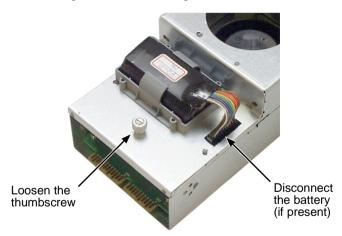
4. If there is a battery on the cooling unit, disconnect the battery connector (above).
